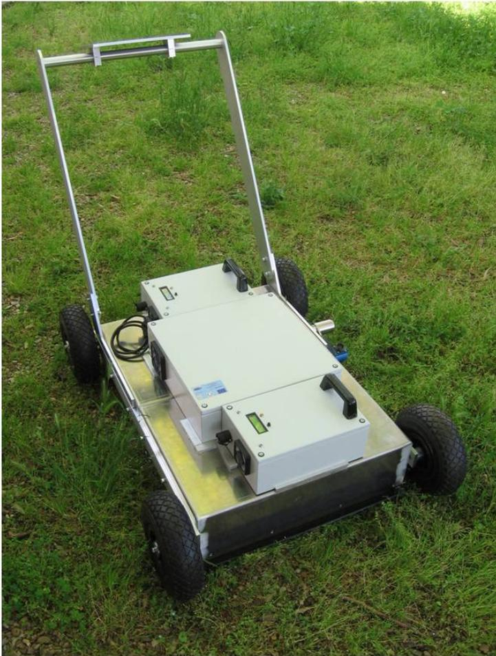
**Three equivalent antennas with the same gap.**
