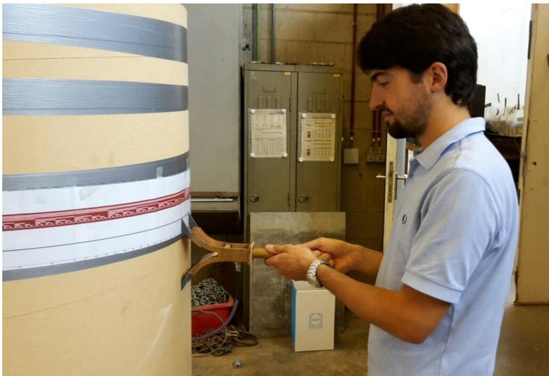
**FIG. 9** – Measurements around the circular cylinder with void inclusion.
