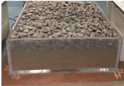
**FIG. 1** – Fouled condition of ballast in the tank at the beginning of the laboratory experiments.
