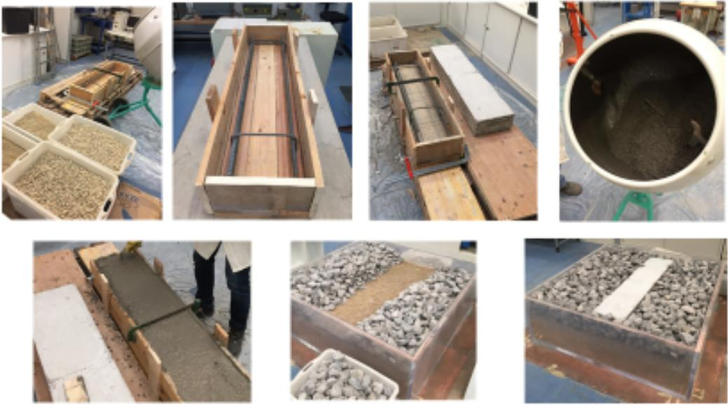
**FIG. 2** - Preparation of sleepers and placing them in the tank.
