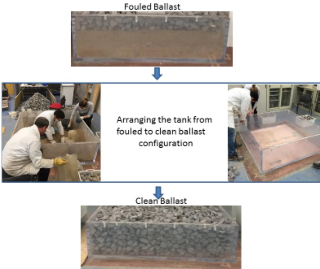
**FIG. 7-** Fouled ballast configuration, arrangement of the tank for clean ballast configuration and finally clean ballast configuration.
