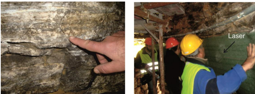
Figure 1 – Data acquisition. Left: Sample of the anomalous surface with a fissure. Right: Laser to produce the circular profiles.
