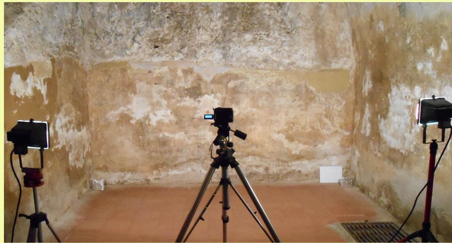
Figure 6: Multispectral data acquisition. Multispectral modified camera in the middle; two halogen lamps symmetrically positioned on the left and on the right.
