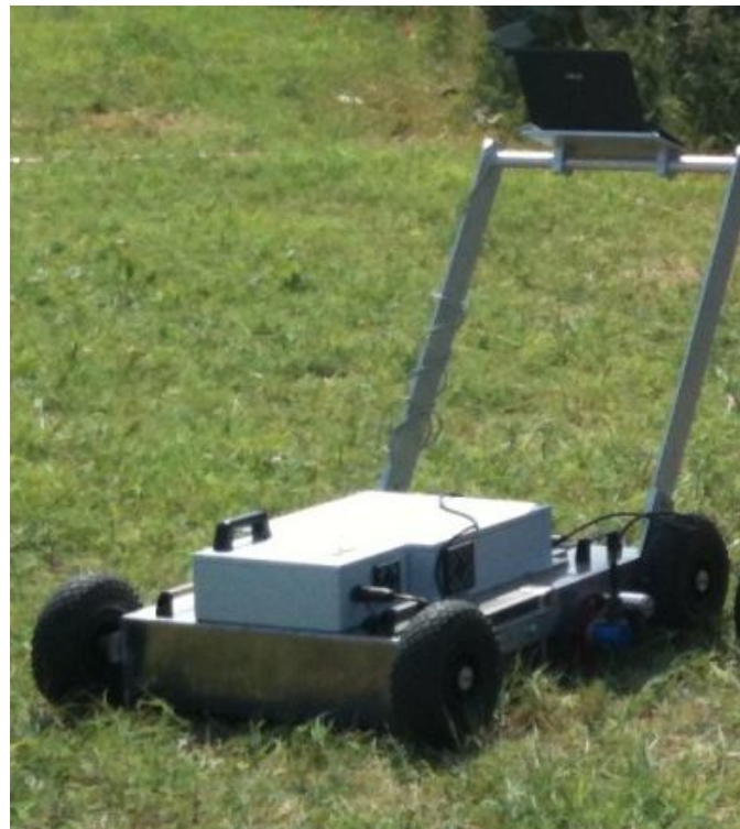
FIG. 6 – Prototypal stepped frequency reconfigurable GPR, built within the AITECH project.
