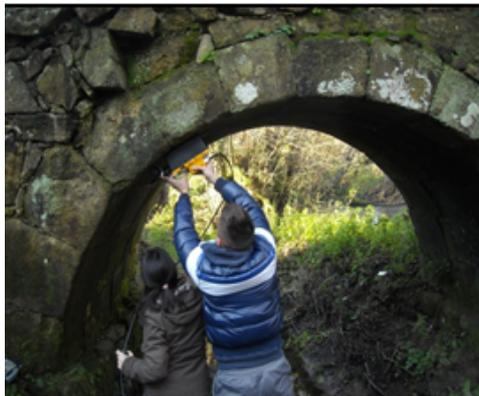
**FIG. 12** – 1-GHz GPR data acquisition through the intrados of the vault arch.
