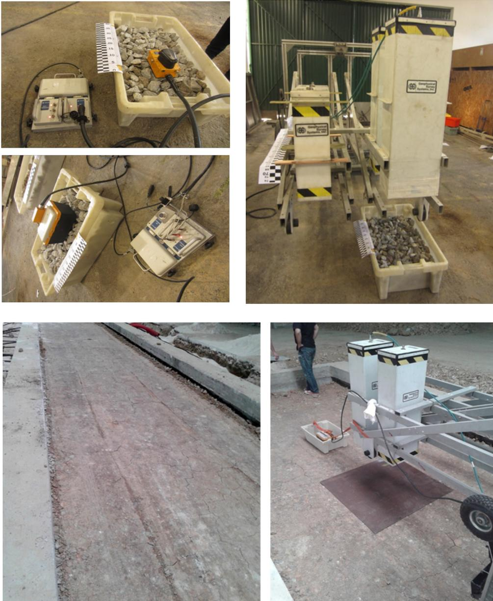
**FIG. 1** – Photos showing the test site at LNEC and GPR data acquisition with ground- and air-coupled antennas.
