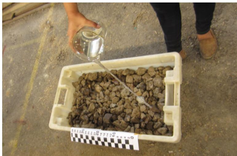
**FIG. 7** – Introduction of water in the specimens.
