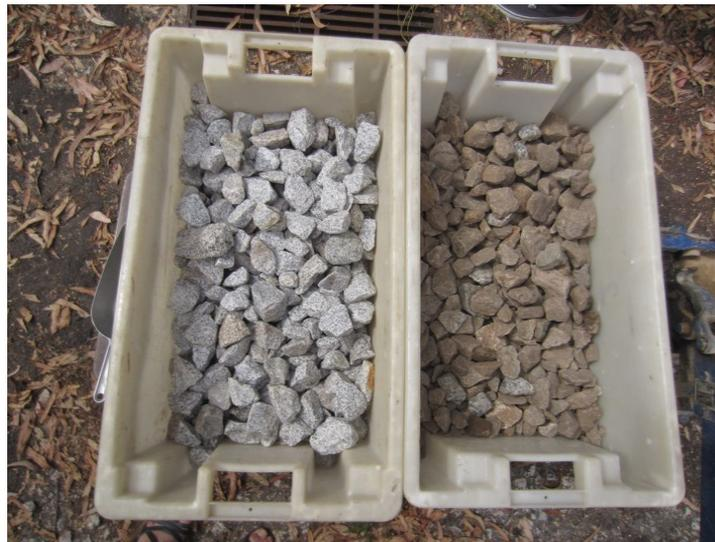
**FIG. 5** – Boxes containing new (left) and used (right) ballast.
