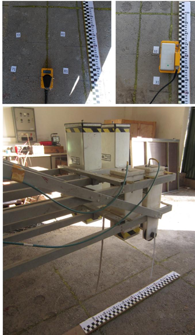
**FIG. 10** – Data acquisition. Upper panel: ground-coupled system with 1.0 GHz (right) and 2.3 GHz (left) antennas. Lower panel: air-coupled system with 1.0 GHz and 1.8 GHz antennas.
