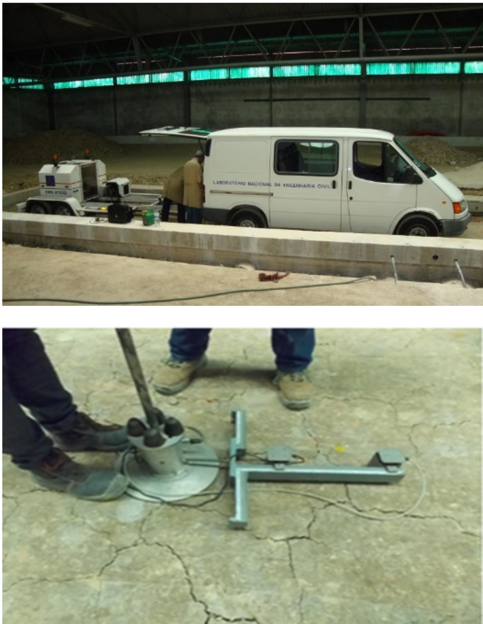
**FIG. 8** – Upper panel: Portable FWD. Lower panel: LFWD.
