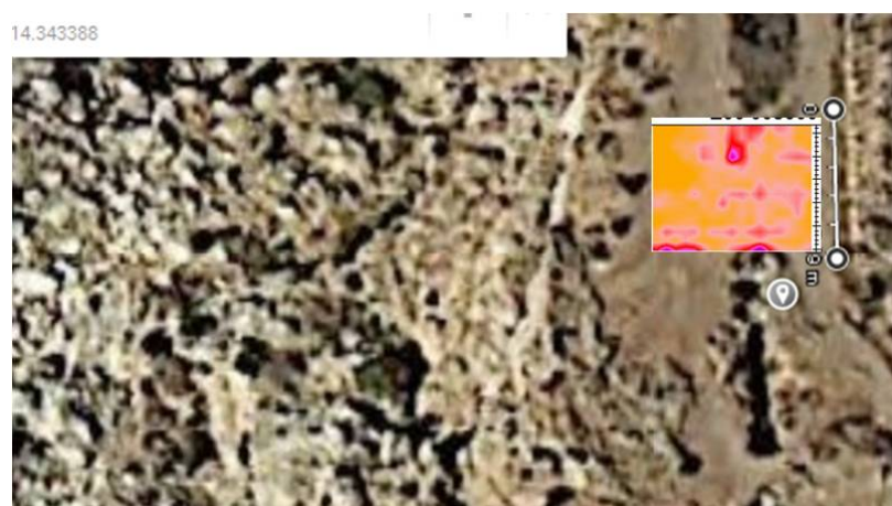
FIG. 5 – Horizontal slice at 15 ns, corresponding to a depth of about 85 cm.
