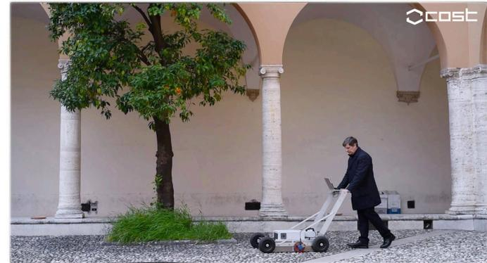
**Project 1.1** Design, realization and optimization of GPR equipment for the monitoring of critical transport infrastructures (pavements, bridges and tunnels)
