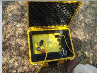
The digital seismograph DAQLINK III of GEOSERVICE was used
