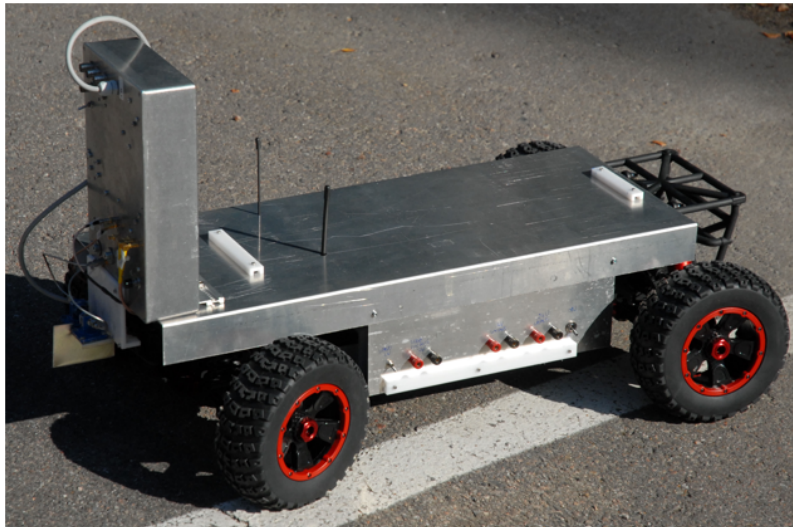
Figure 4. Ready asphalt radar rover on the street. The two monopole antennas are for vehicle telecommand and for radar telemetry. Radar antennas point towards the road in the front of the car.
