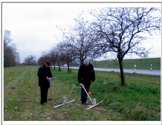
Fig. 4. Field operation with Loza-V GPR.
