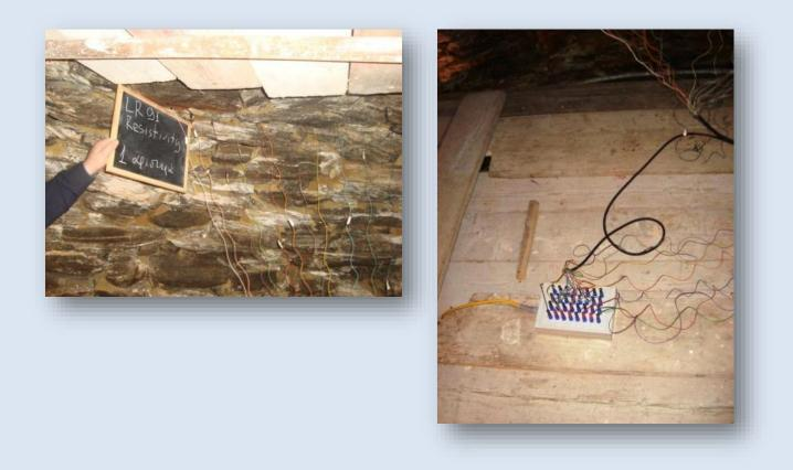
Type of spread: 32 Electrodes multi electrode configuration. Schlumberger – Wenner arrangement.
